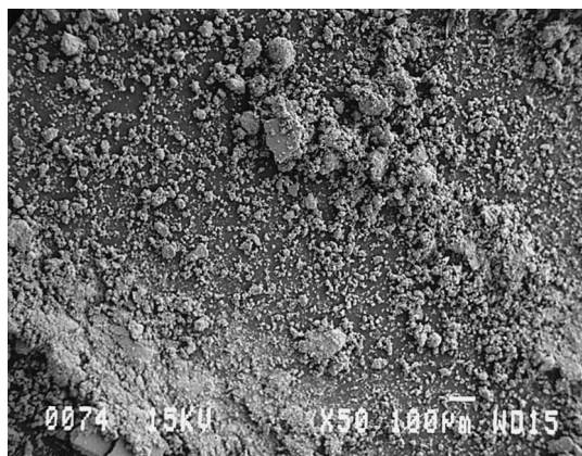
Fig. 8. SEM photograph of (\text{UO}_3 + 3\text{C})^* ground mixture; magnification \times 50 .
